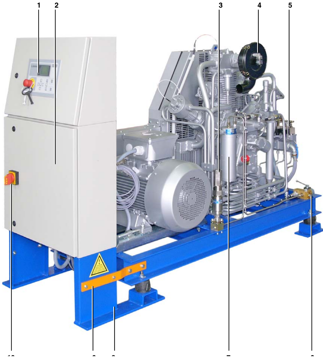
Fig. 1 Breathing air compressor unit; shown: KAP 22.0, standard version
